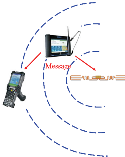
Fig. 5. Eavesdropping on reader-tag communication
